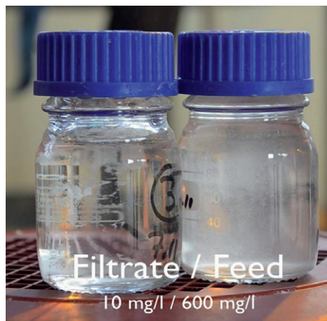
Figure 2: Clear process water produced by the Sofi Filter.
